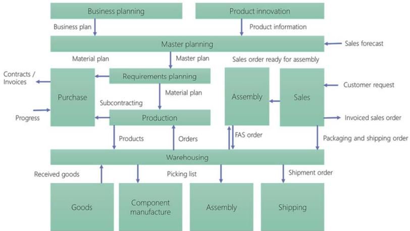
Fig. 2.21. An Example of the Data Flow in the ERP architecture
