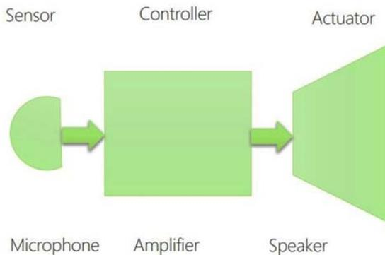
Fig. 6.8. Sensor – Controller – Actuator Example
