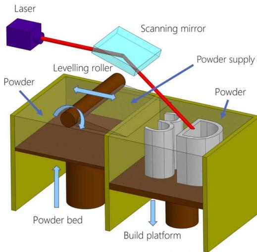
Fig. 6.22. SLM 3D Printing
