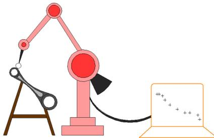
Fig. 2.42. Contact Scanning
