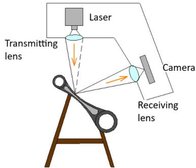
Fig. 2.41. Non-contact Scanning
