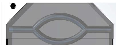
Fig. 2. The shape of the reinforcing elements of the bed
