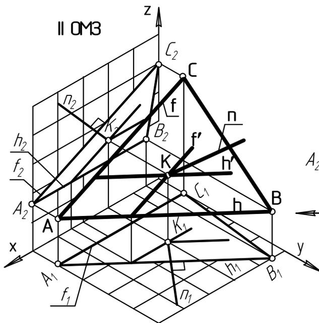
$$n \perp f \wedge n \perp h \Rightarrow n \perp \Gamma(f \cap h)$$
