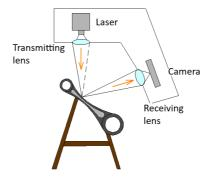
Fig. 2.41. Non-contact Scanning
