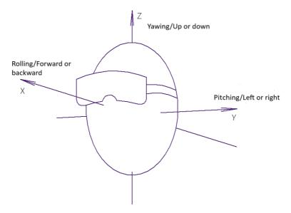
Fig. 2.50. Degrees of Freedom of a VR Device
