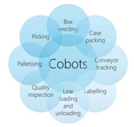
Fig. 6.5. Cobot Functions
