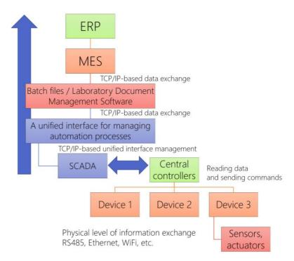
Fig. 2.19. Data Structure in SCADA
