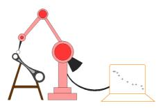
Fig. 2.42. Contact Scanning
