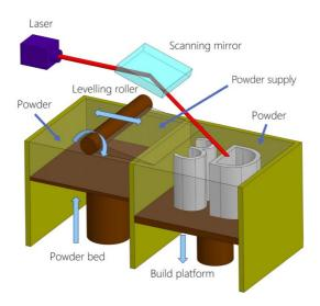
Fig. 6.22. SLM 3D Printing
